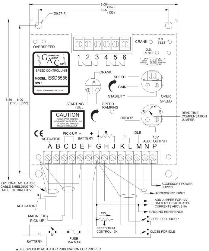
WIRING OF ACTUATOR BASED ON BATTERY VOLTAGE
